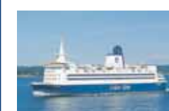
M/S COLOR VIKING Sandefjord - Strömstad Year built: 1985 Register: NOR Tonnage: 19 763 BRT Length: 137 metres Max. speed: 18 knots Passenger capacity: 1 720 Cabins: 0 Berths: 0 Freight capacity (lane metres): 490 Vehicles: 370
