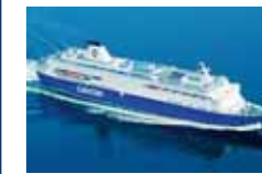
M/S PRINSESSE RAGNHILD Bergen/Stavanger-H.hals Year built: 1981/1992 Register: NOR Tonnage: 35 855 BRT Length: 205,3 metres Max. speed: 21 knots Passenger capacity: 1 515 Cabins: 566 Berths: 1 766 Freight capacity (lane metres): 900 Vehicles: 650
