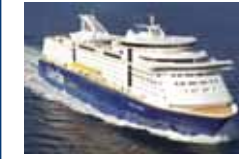
M/S COLOR FANTASY Oslo - Kiel Year built: 2004 Register: NOR Tonnage: 75 027 BRT Length: 223,7 metres Max. speed: 21 knots Passenger capacity: 2 750 Cabins: 966 Berths: 2 799 Freight capacity (lane metres): 1 270 Vehicles: 750
