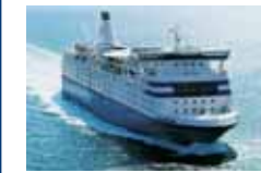
M/S COLOR FESTIVAL Oslo - Frederikshavn Year built: 1985 Register: NOR Tonnage: 34 694 BRT Length: 171,5 metres Max. speed: 21 knots Passenger capacity: 2 000 Cabins: 568 Berths: 1 909 Freight capacity (lane metres): 800 Vehicles: 330
