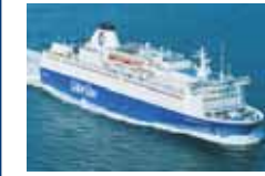
M/S KRONPRINS HARALD Oslo - Kiel Year built: 1987 Register: NOR Tonnage: 31 914 BRT Length: 166,3 metres Max. speed: 21 knots Passenger capacity: 1 458 Cabins: 480 Berths: 1 458 Freight capacity (lane metres): 1 000 Vehicles: 750
